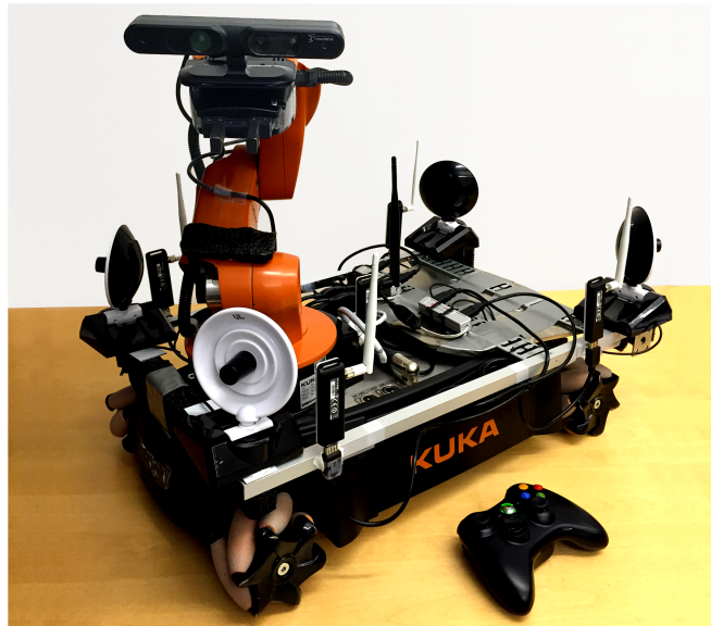
Fig. 1: A youBot mobile robot equipped with wireless network hardware used in the experiments. The directional antennas are visible in the corners of the youBot, and the omnidirectional antenna for communication in the center.
